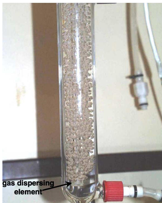
Fig. 3. Picture of the lower part of the stripping cell. It shows the gas-dispersing element releasing gas bubbles at the bottom of the solution. The bubbles rise through the solution and equilibrate with dissolved VOCs, during their residence time in the solution.
